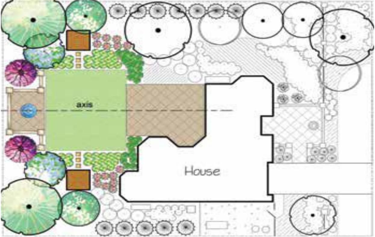
figure 12. Symmetrical balance around an axis
