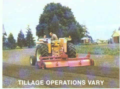
Fig. 1—Rotary Tillers are Used for many Tillage Operations
