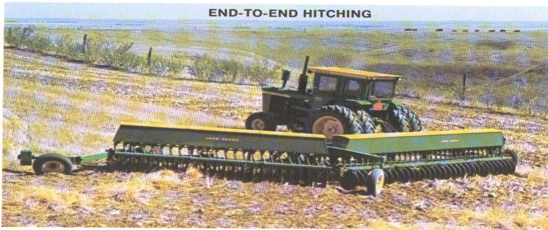
Fig. 36—End-to-End Hitching with Ball-and-Socket Coupling
