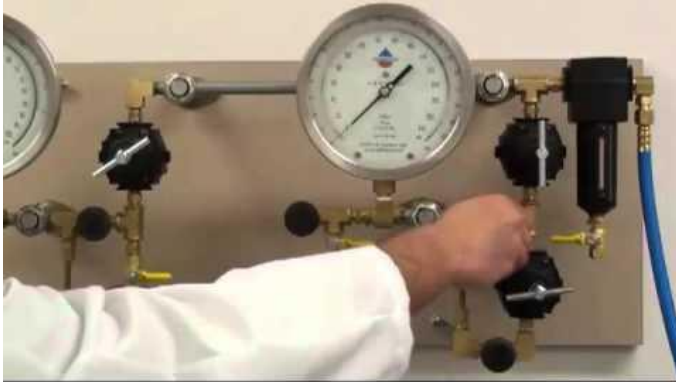
Open the coarse Regulator Valve to place the Gauge in line with the Coarse Regulator.
