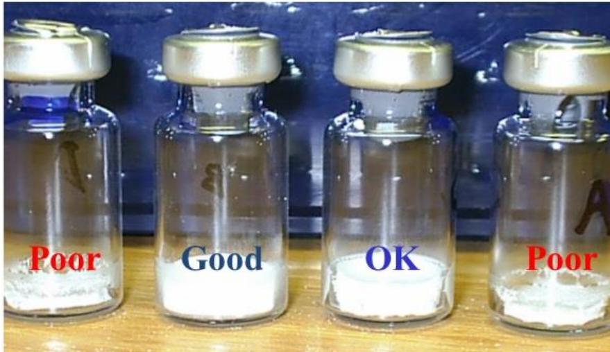
The product in the "Poor" vials has become soft and dense during freeze-drying, because it has become warmer than its "Critical Temperature"
